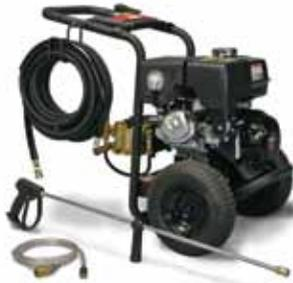
**The DA Series** is a rugged, yet compact, line of direct-drive cold water pressure washers. Powered by Honda GX or GC engines, the DA series delivers cleaning power up to 3500 PSI with an all-welded chassis protected with all-weather, epoxy powder coat finish. The Hotsy triplex pumps carry a 7-year warranty. 5 HP models equipped with a 25' hose; 6.5 & 13 HP models equipped with a 50' hose.
